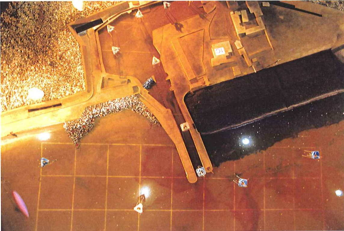
Plate 20a Erosion of the beach at the existing East Pier, waves from 220°N, pre-test
