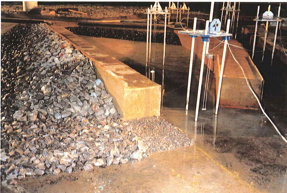
Plate 15 Construction phase tests, close-up of temporary works, Test Series 7a
