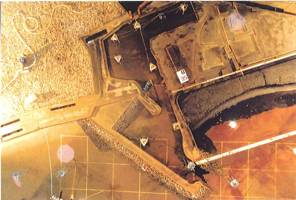
Plate 21c Erosion of the beach at the extended East Pier, waves from 220°N, prototype test duration 42.8 hours
