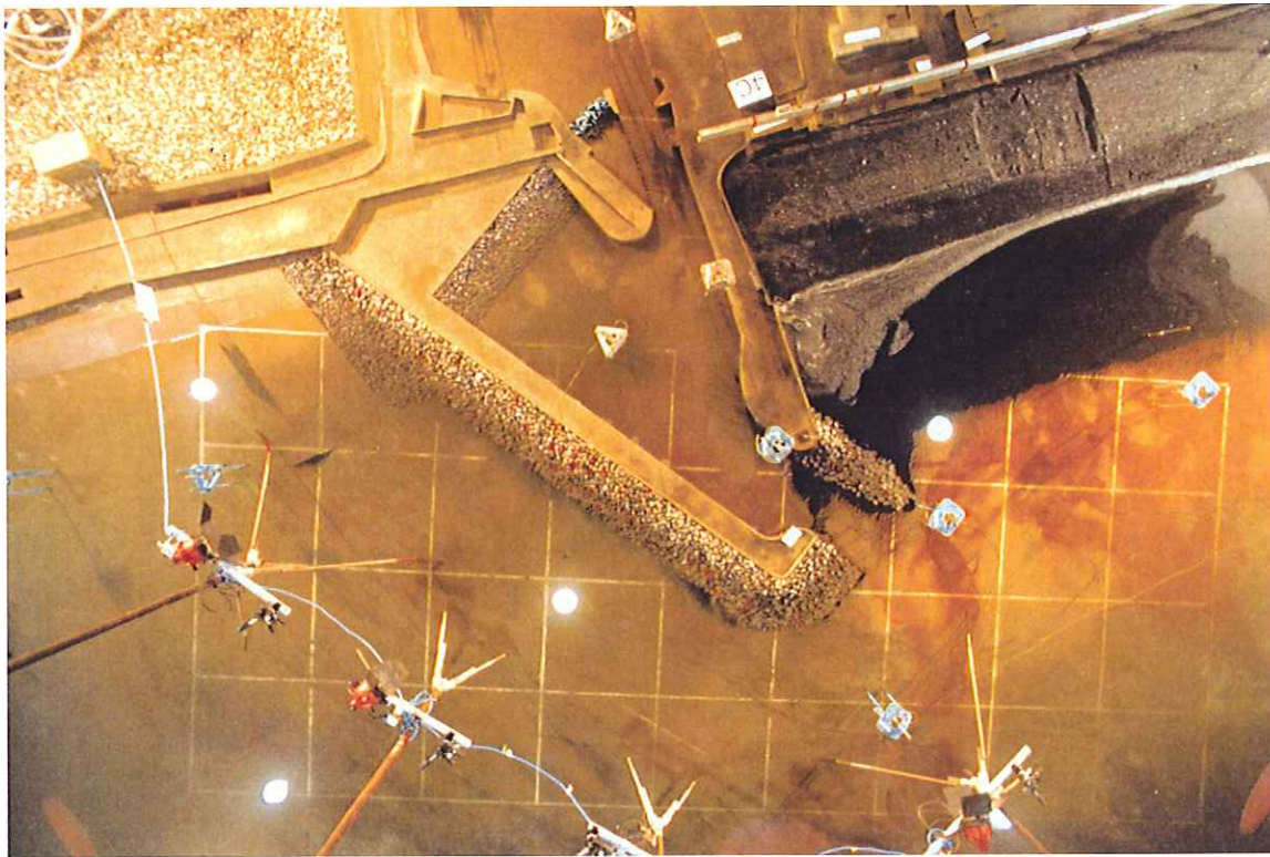
Plate 19a Accretion of the beach at the extended East Pier, waves from 160°N, prototype test duration 31.8 hours
