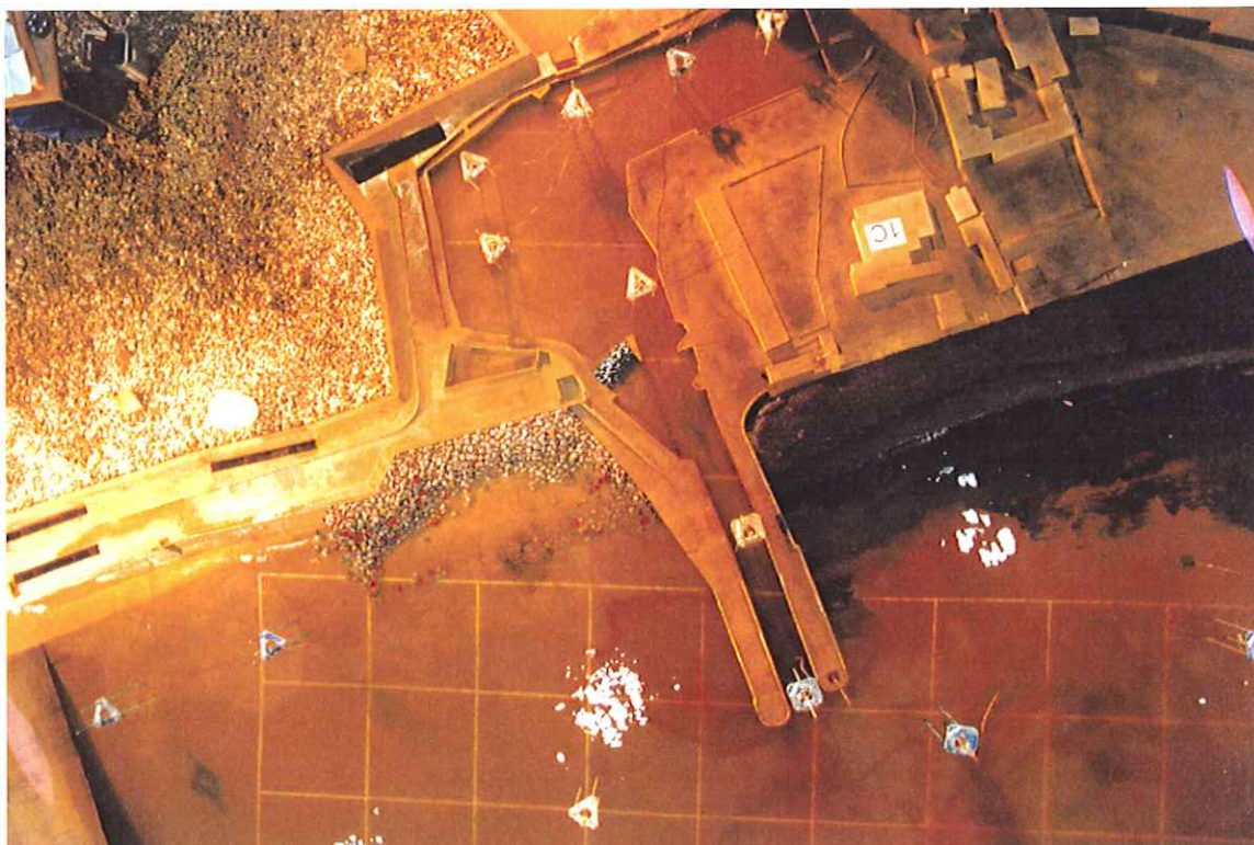
Plate 20b Erosion of the beach at the existing East Pier, waves from 220°N, prototype test duration 20.5 hours
