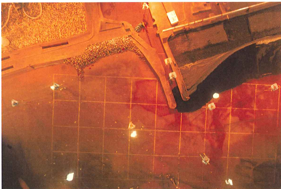
Plate 18d Accretion of the beach at the existing East Pier, waves from 160°N, prototype test duration 58.3 hours
