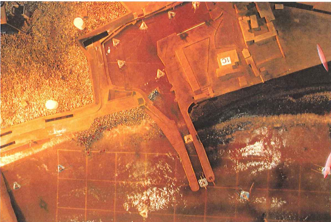
Plate 20d Erosion of the beach at the existing East Pier, waves from 220°N, prototype test duration 89.4 hours
