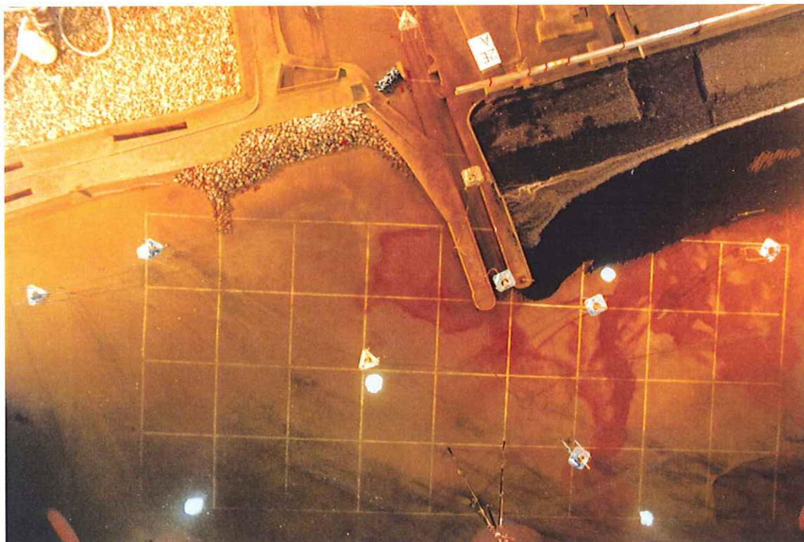
Plate 18b Accretion of the beach at the existing East Pier, waves from 160°N, prototype test duration 14.6 hours
