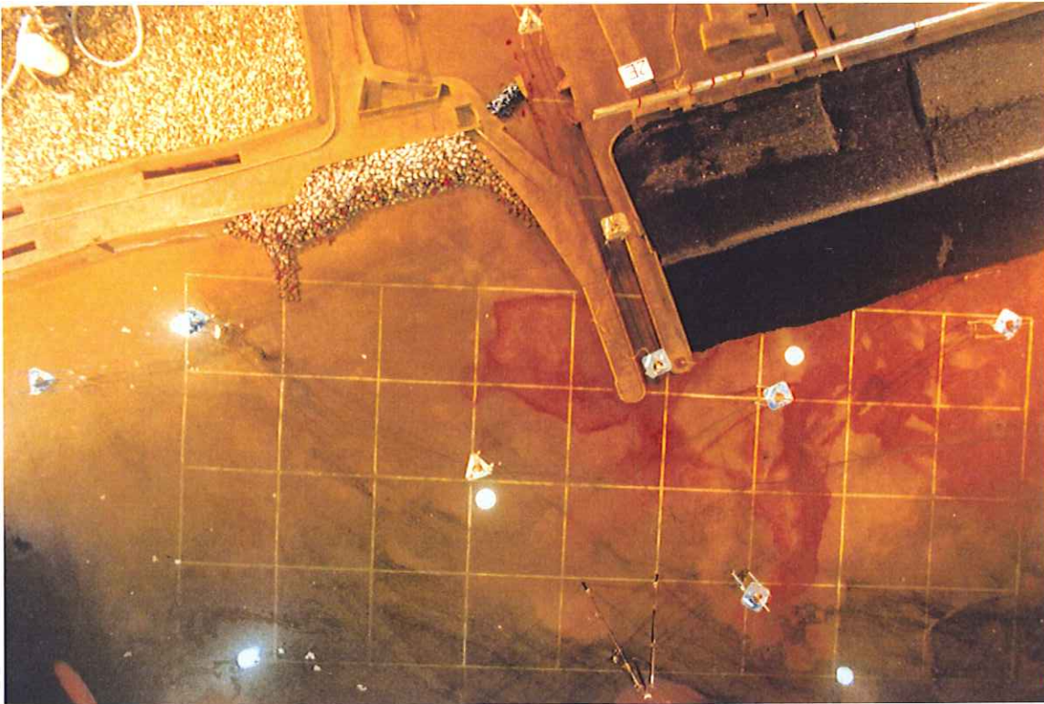
Plate 18a Accretion of the beach at the existing East Pier, waves from 160°N, pre-test
