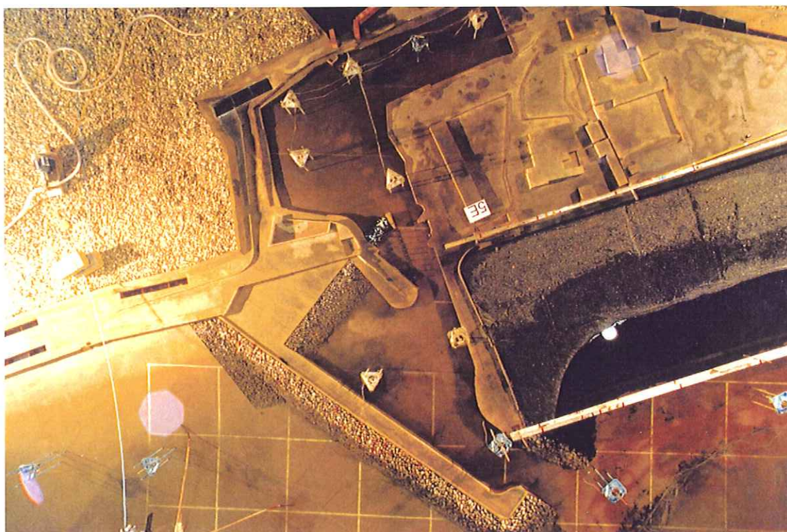
Plate 21a Erosion of the beach at the extended East Pier, waves from 220°N, pre-test
