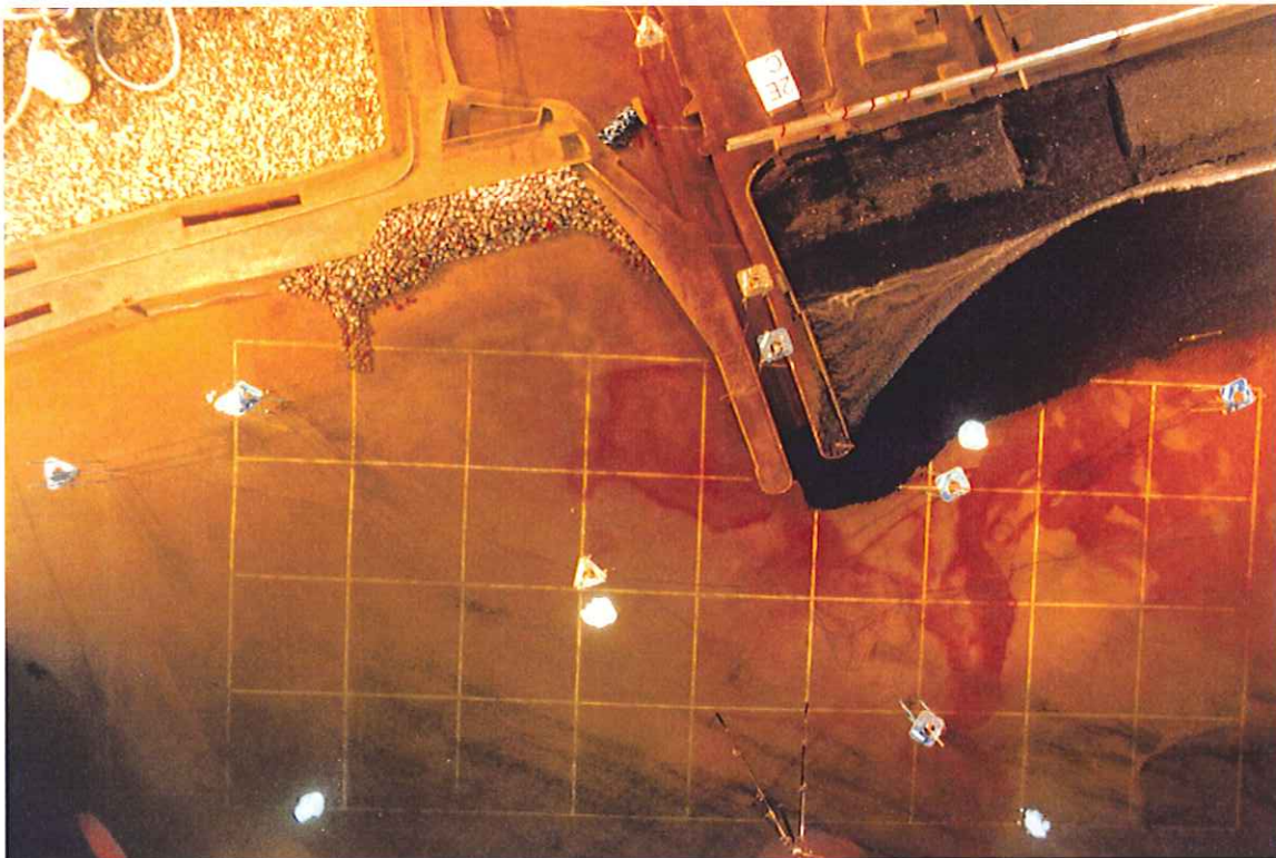
Plate 18c Accretion of the beach at the existing East Pier, waves from 160°N, prototype test duration 43.7 hours
