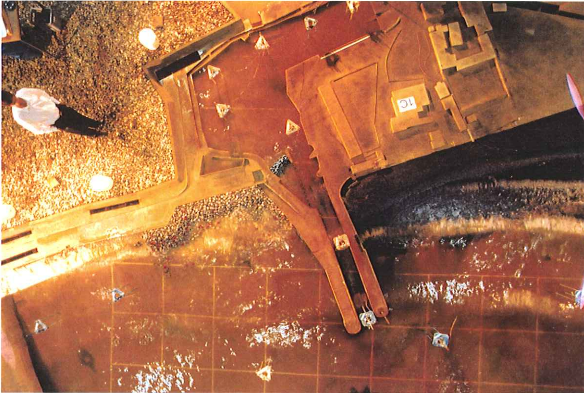
Plate 20c Erosion of the beach at the existing East Pier, waves from 220°N, prototype test duration 57.3 hours
