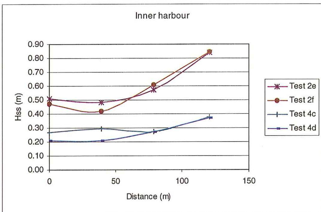
Figure 27 A comparison of wave heights within the harbour, 1:1 and 1:10 year condition, waves from 160°N, existing and layout assessed during Test Series 4
