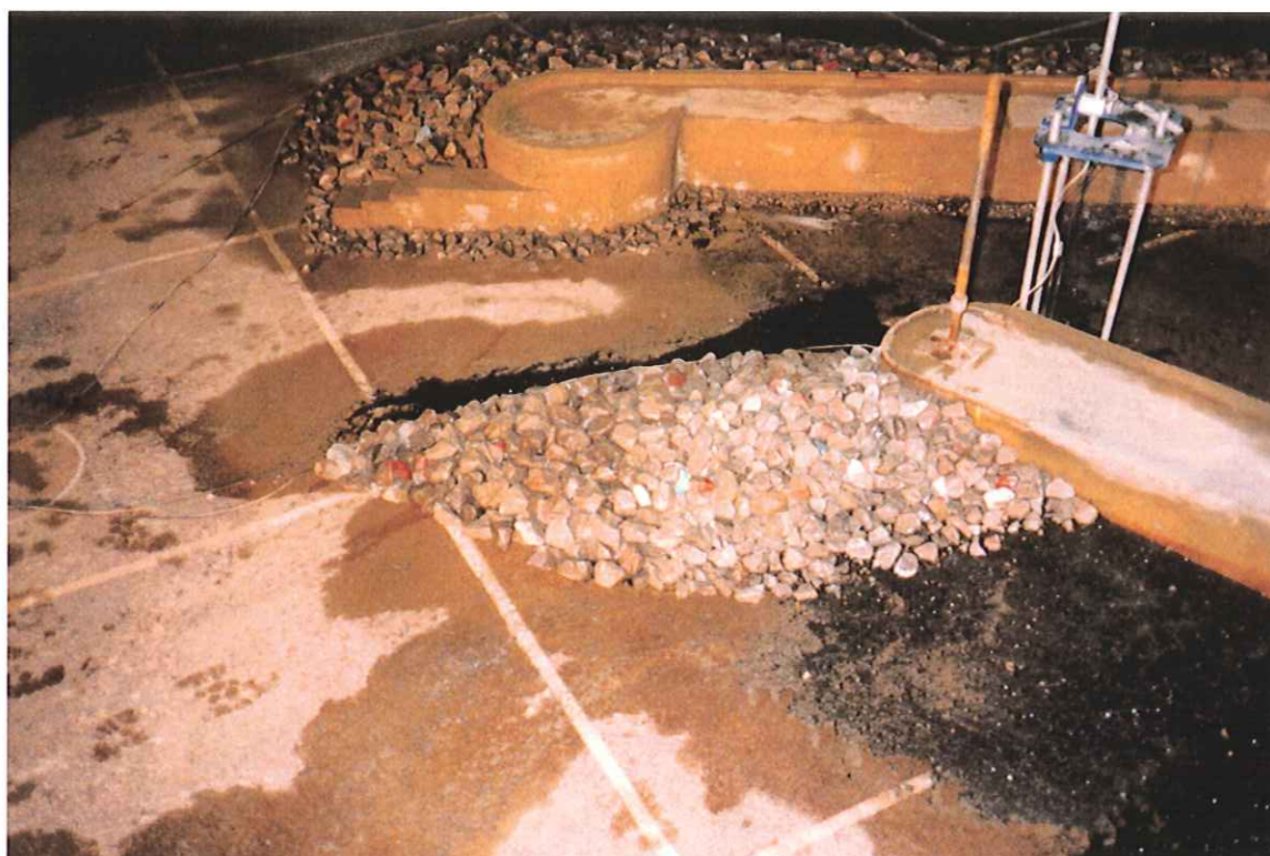
Plate 13b Roundhead and East Pier extension detail after Test Series 6
